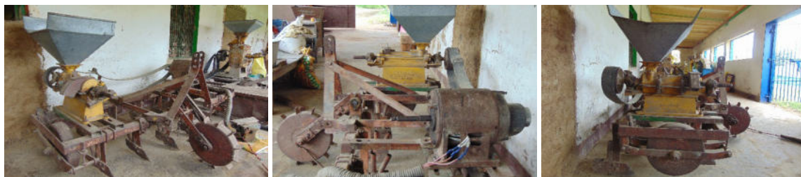
Fig 7.4 : Farmer's innovation: Movable rice huller on non-functional ZT machine
