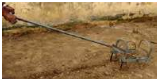
Fig. 4.14. Prototype of the manual weeder
