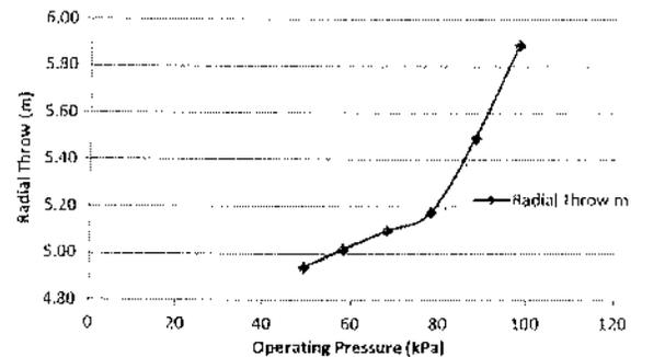
Fig. 13 Radial water distribution pattern of wobbler at varying operating pressure
