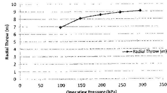
Fig. 10 Radial water distribution pattern of single nozzle impact sprinkler at varying operating pressure
