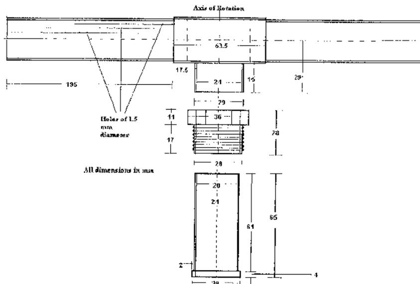
**Fig. 2** Configuration of developed LEWA device**Fig. 3** Head discharge relationship of LEWA device
