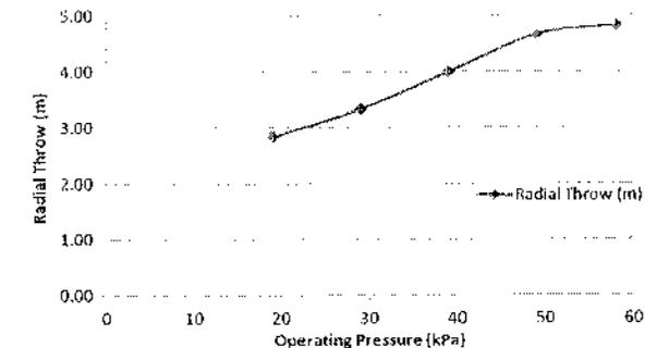
Fig. 5 Radial water distribution pattern of LEWA at varying operating pressure
