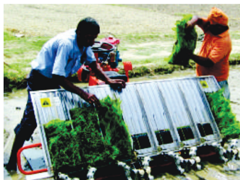
Mat nursery tray of self propelled Mechanical rice transplanter
