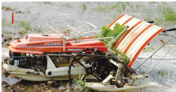
Mechanical rice transplanter (Manually operated)
